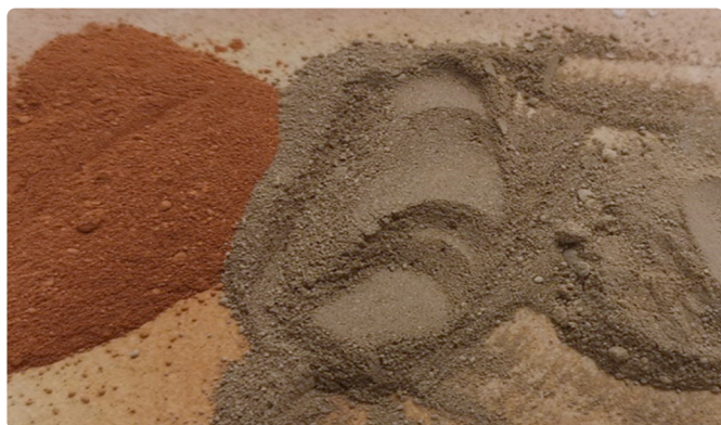
Colour control with flash calciner Comparison with and without colour control
