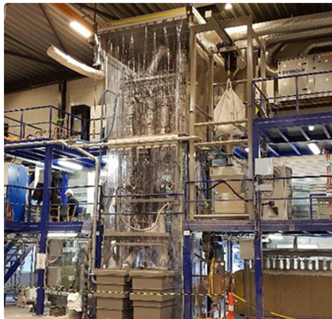
Pilot Installation for SCM pyroprocessing - At FLSmidth Cement's R&D Center Dania, Denmark
